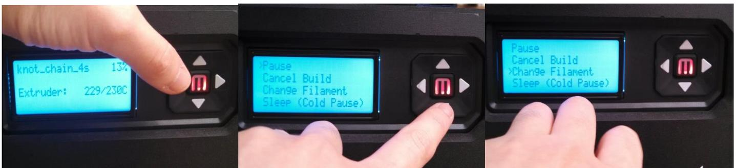
This will pause the print, move the extruder out of the way, and give you time to assess the situation. If done quickly enough, you can even recover a print that would have otherwise failed.
